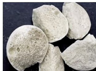
Structural LiGrA Densely packed finer pores
