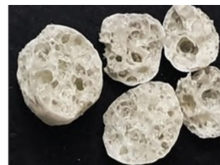
Non-Structural LiGrA Loosely packed coarser pores
