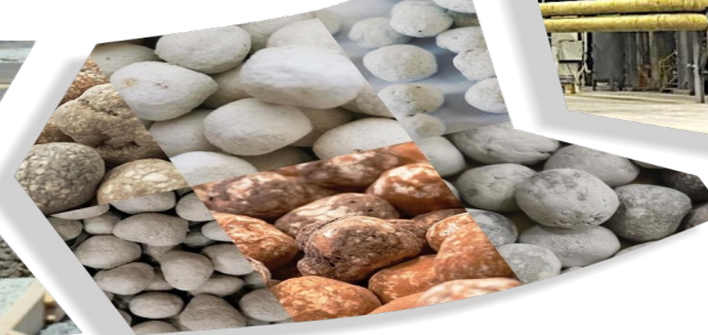
Various Lightweight Green Aggregates (LiGrA)
