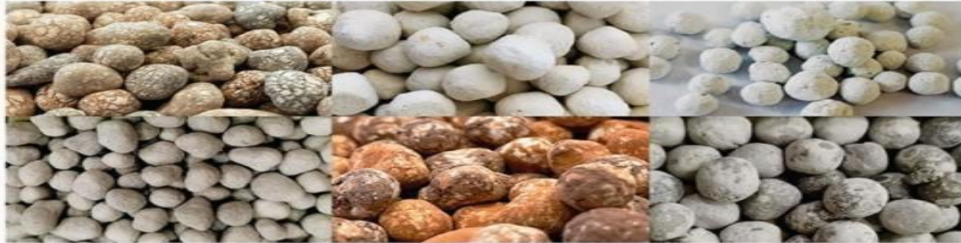
Joe Green's Lightweight Green Aggregates (LiGrA) building materials (above) are made from recycled waste. PHOTO: JOE GREEN
