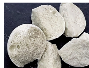
Structural LiGrA Densely packed finer pores
