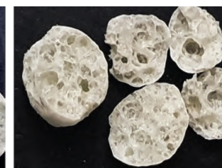
Non-Structural LiGrA Loosely packed coarser pores
