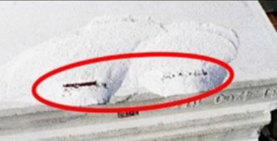
Porous, Corrodes BRC inside, Bending and No Strength
