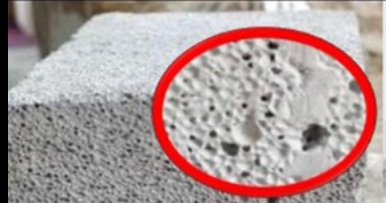
Porous, Corrodes BRC inside, Bending and No Strength
